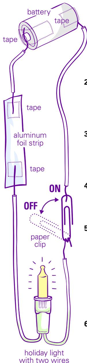
1. Tape one end of each stripped wire to each end of the battery, so the bare wire touches the center of each end of the battery.
