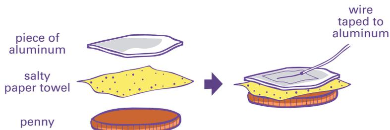
3. Make three more sandwiches and stack them beneath the first penny with the wire taped to it.
